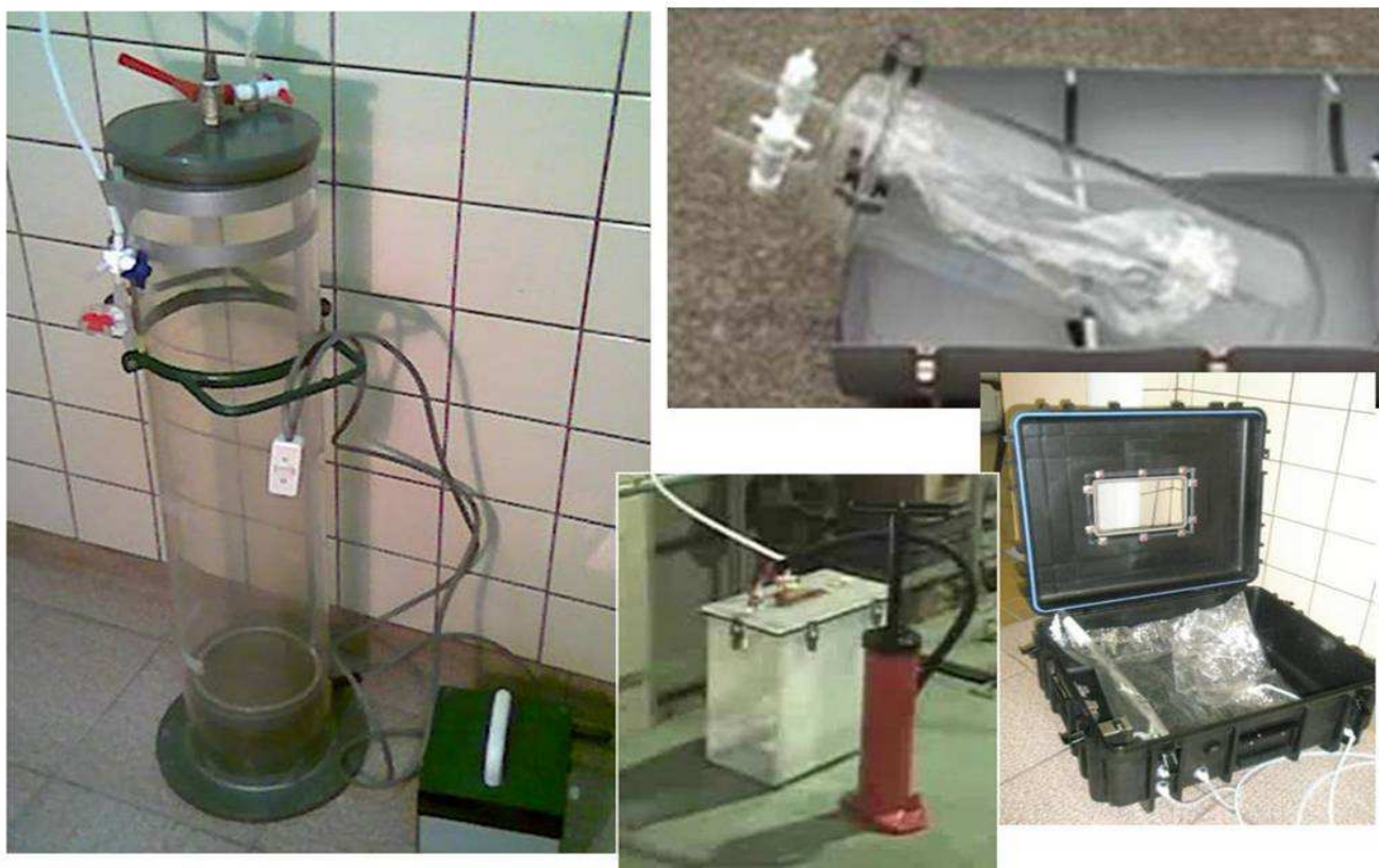
Fig. 2. Collecting samples with "The lung principle"
