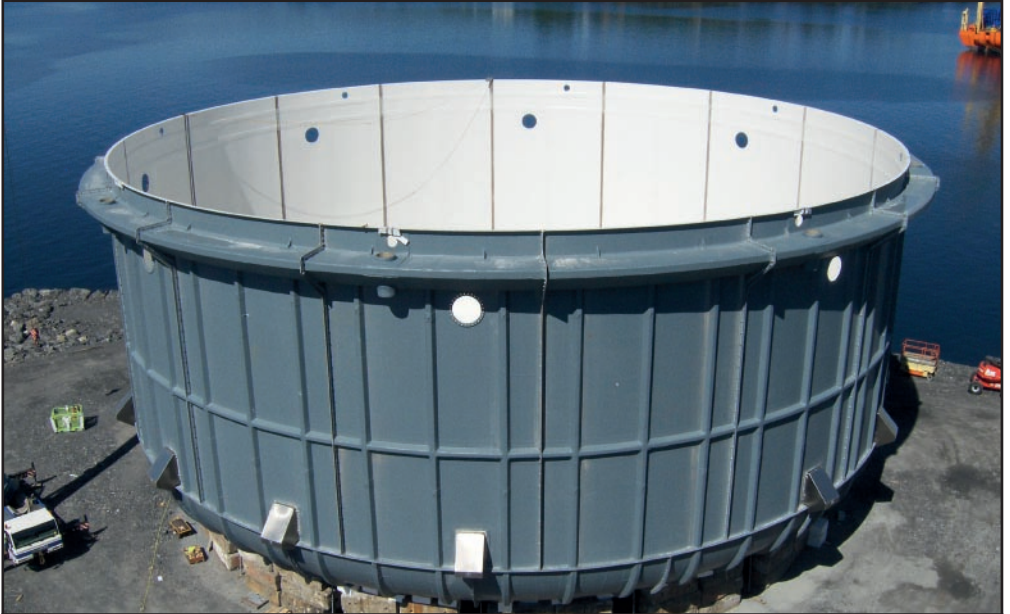
Figure 14: Aquafarm Equipment’s new closed cage for aquaculture is being tested in full scale. Researchers shall monitor the fish health, water quality and optimize the temperature, oxygen concentration, and water flow. Also the mechanical and structural parts of the system shall be tested thoroughly.
